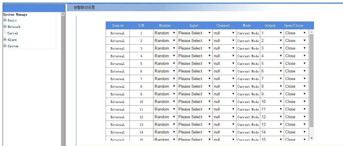
[Figure 4-48] Alarm linkage setting
